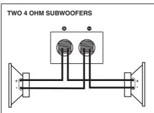
NOTE! Two 4 ohm subwoofers gives a 2 ohm load when connected in this way. The minimum amplifier load is 1 ohm, lower impedances may damage the amplifier!
