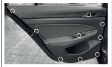
Usually the clips/screws are placed by the white marks. This could vary depending on the vehicle.
