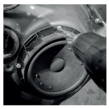
Drill just enough to remove the top of the rivets, and the speaker will come loose.
