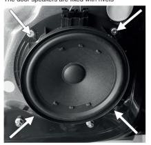
Use a 4mm drill bit to remove the rivets. Make sure all remains from the old rivets are removed from the inside of the door.
