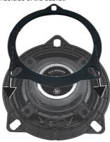
Mount the foam gasket (115mm x 4mm) on the top of the basket. Peel off the protective cover of the self adhesive tape. Press firmly all around so that the foam gasket sticks thoroughly.
