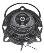
Mount the foam gasket (115mm x 13mm) on the top of the basket. Peel off the protective cover of the self adhesive tape. Press firmly all around so that the foam gasket sticks thoroughly.
