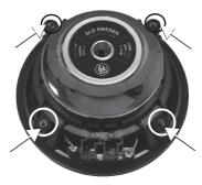
Place the plastic frame over the speaker and fix the frame with four included screws.
