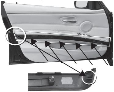
Remove the T20 screws. You need to remove the door handle as well, if the panel is equipped with one. Use PRY tool and be careful. T20 screw at the top of the handle and in some models a screw at the bottom of the handle.
