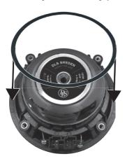
Remove the centerpiece of the small ring of the EVA gasket. This piece will not be used. Use a narrow tool to pick up the small ring from the same EVA gasket.
