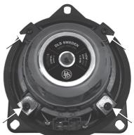
Mount the EVA gasket (102mm x 1.5mm) on the underside of the basket. Peel off the protective cover of the self adhesive tape. Press firmly all around so that the EVA gasket sticks thoroughly.
