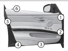
Remove the door panel. Start on the inside. Use a PRY tool. Insert the PRY tool behind the panel and carefully bend the tool towards you. If your car has a lock pin (6), make sure to remove it before lifting the door cover.
