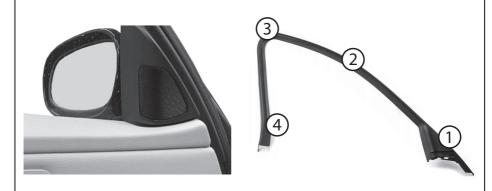
Remove the soft inside cover to find the tweeter. Gently press out the "hooks" to loosen the tweeter. Unplug the tweeter harness.
