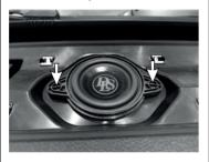
Install the speaker cover by pressing it down and make sure that all clips engage.
