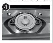
The center speaker is "locked" with plastic plugs, lever the speaker upwards with the Pry tool.
