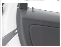
Some newer models don't have plastic clips to hold the door in place. Just remove the screws and gently press the door panel up. Be careful with the door lock knob. Just move the panel straight up.
