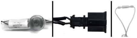
The yellow cable loop is tweeter level select, enabling fine tuning of the high frequencies Closed loop = -4de (Shown in the picture)
