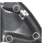
Attach the 3M double-sided adhesive tape to the sound optimized tweeter bracket. Mount the new DLS tweeter in the bracket. Remove the protection plastic from the 3M tape and place the bracket in the OEM tweeter cover. Press the bracket down, to attach to the OEM tweeter cover.
