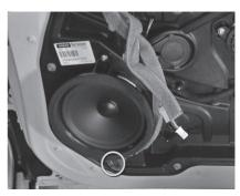
Hint: Don't forget to connect the tweeter cable (with crossover) to the OEM harness, before reassembling the door panel. The crossover needs to be placed behind the door panel. Use foam pads to wrap cables/crossover to prevent rattling.
