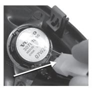
Use a Snap-off blade knife or a cutting nipper to remove the top of the plastic pin that holds the OEM-tweeter. When the tweeter is dismounted, make sure to remove all material from the pin that was used to fix the OEM-tweeter.
