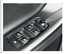
Remove the electric window panel and disconnect the plug on the back side of the panel. Always use plastic PRY tools when removing panels and interior, to avoid marks on the panels and leather.
