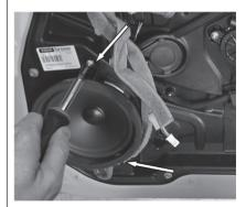
Connect the speaker harness. Start the assembly of the door panel. Reconnect all wires harness.
