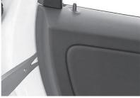
Some newer models, don't have plastic clips to hold the door in place. Just remove the screws and gently press the door panel up. Be careful with the door lock knob. Just move the panel straight up. There are several electric and mechanical connectors on the backside of the door panel. Release the door lock cable.
