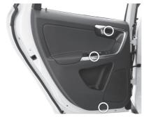
Be careful when removing the door panels and lids. Use PRY tools.
