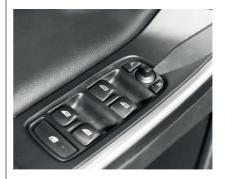
Remove the electric window panel and disconnect the plug on the back side of the panel. Always use plastic PRY tools when removing panels and interior, to avoid marks on the panels and leather.
